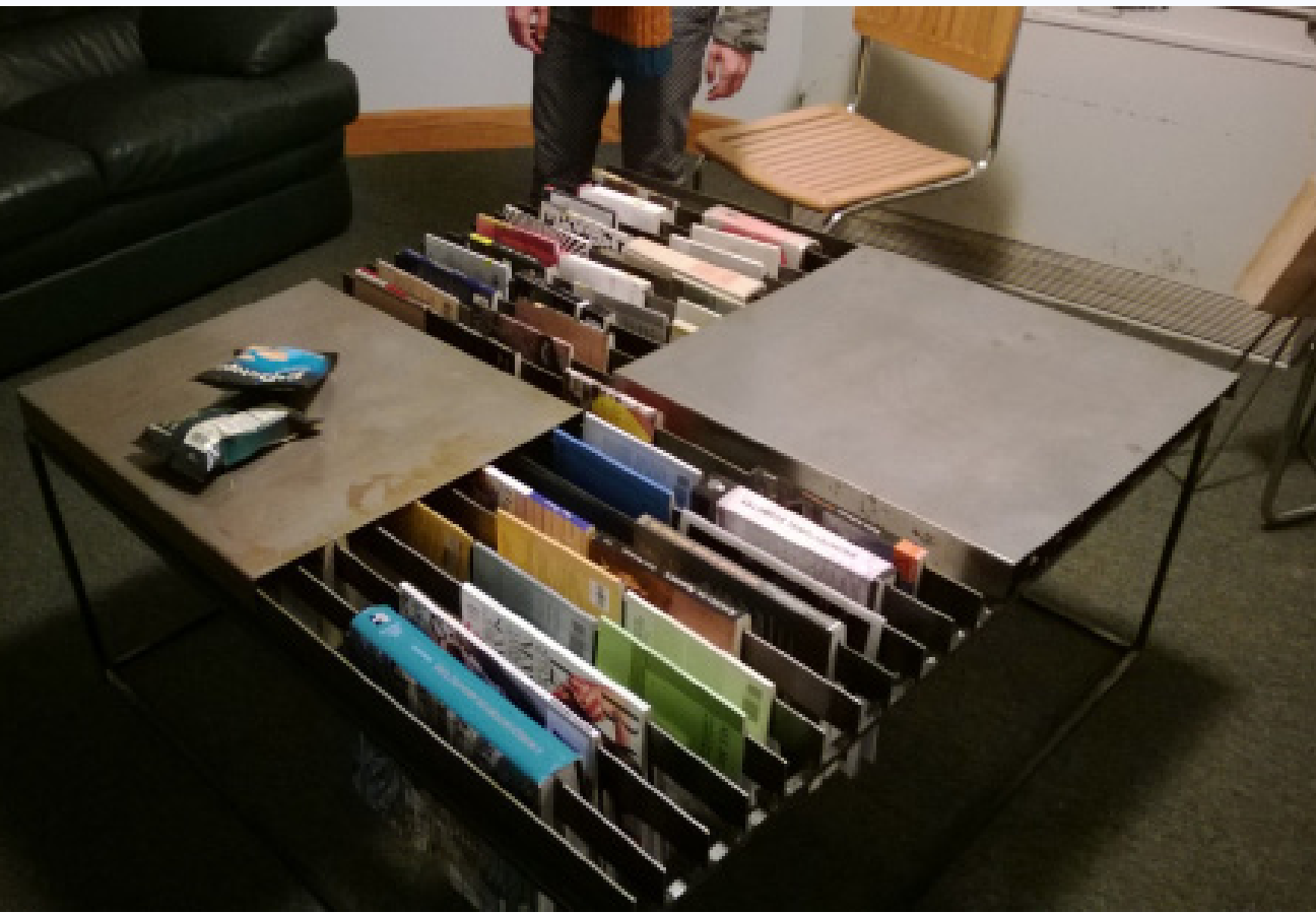
bookshelf with sliding surfaces, steel barstock, metal brake, varnish, mig welder
